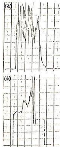
Fig. 3 (a) RPA Data EBA : 2kV Transient Record (10V, 2µs)
