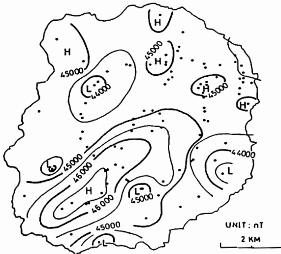
Fig.1 Distribution of smoothed total force intensity surveyed on the ground. Contour interval is 500 nT.
