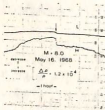
Fig. 1. Change in the resistivity at the time of an earthquake of magnitude 8.0 on May 16, 1968 as recorded by high (H) and low (L) sensitivity channels. The epicentral distance amounts to 680 km.
